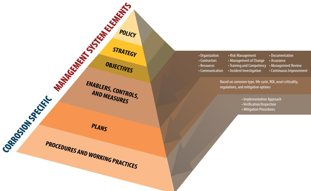
Figure 2. The CMS Pyramid: Hierarchy of general and corrosion-specific management elements.
