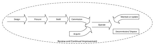
Figure 3-5. Corrosion Management over the Life Cycle of the Asset
