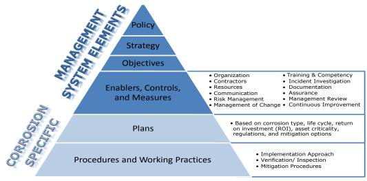
Figure 7-1. The Corrosion Management System Pyramid
