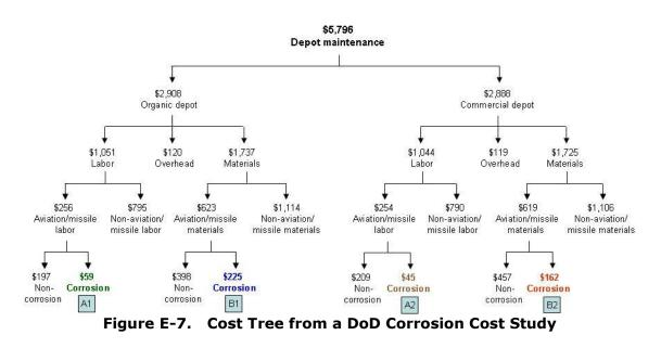
The cost diagram in Figure E-7 outlines the spending on corrosion during depot maintenance of a military aircraft<sup>46</sup>. The logic and appearance of this diagram is similar to that of the "meat" example with each lower level of the cost tree summing to the level above it. The real challenge here is to conduct the bottom-up analysis – in essence, extracting the corrosion-related costs from the operations and maintenance activities.
