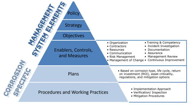
Figure 3-3. Hierarchy of General and Corrosion-Specific Management Elements
