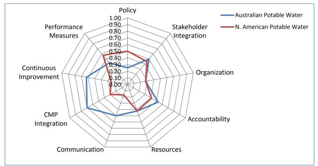
Figure 5-8. Radar Plot Comparing Corrosion Management Practices in Australia and North America
